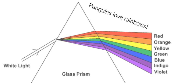
The quantitative measurement of the absorption or transmission properties of a material as a function of wavelength is called **spectrophotometry**, and the instrument we use is called a **spectrophotometer**.
