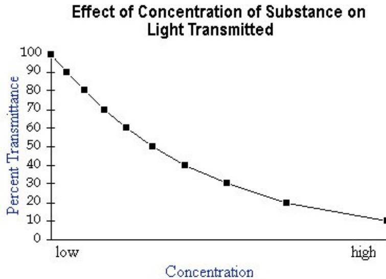
As you can see, the relationship is exponential, which is awkward to work with. The good news is that since transmittance decreases *exponentially* with concentration, *log 1/T increases linearly with increasing concentration!* That's great because straight lines are a lot more convenient than curved ones! Here's a graph of **absorbance** as a function of concentration:
