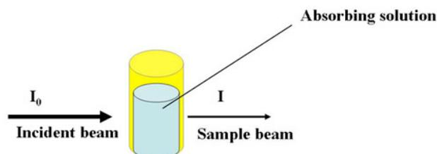
The spectrophotometer measures transmitted light through a sample with respect to the incident light very precisely. Check this out:
