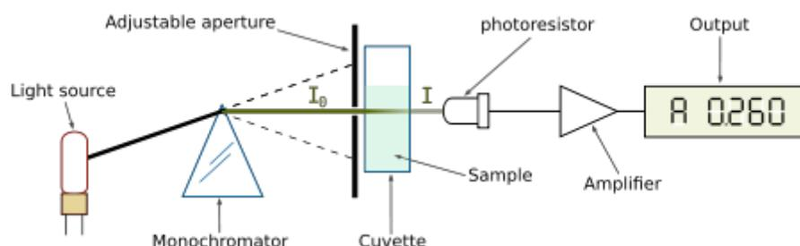
OK. As you can see, the spectrophotometer measures how much light is **transmitted** through our sample (compared to how much light entered the sample). Transmittance is simply the percentage of incident light reaching the photocell:
